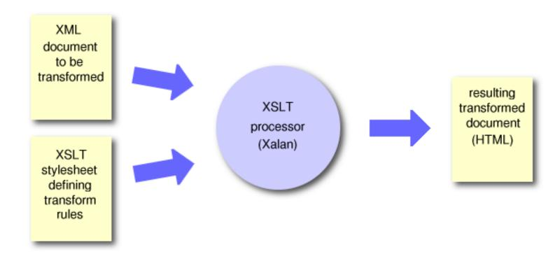
An XSL Transformation processor is a piece of software that takes both the original XML document and an XSL stylesheet as inputs, and produces the resulting transformed document. In the above case, the output format is HTML. There are a number of XSLT processors on the market today, written in many programming languages. One to note is the Xalan processor, which is a robust, open-source processor from <a href="http://xml.apache.org">http://xml.apache.org</a> that is implemented in Java.
