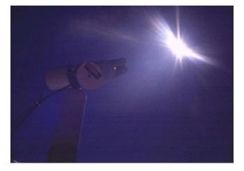
The LTER/NASA Sun Photometer collaboration is part of the larger NASA AERONET sun photometer project at NASA/GSFC. The automated robotic instruments gather data to determine amounts of aerosols, dust and water vapor in the atmosphere. Sun photometers have been in placed at more than 10 LTER sites on a partial or permanent basis starting in 1993.
