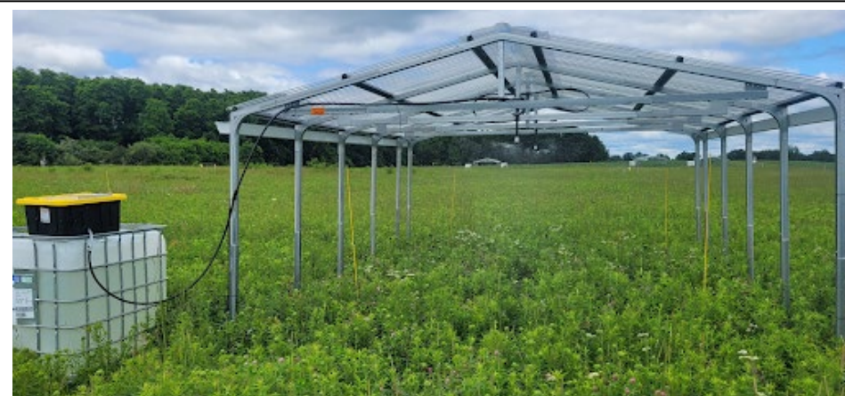
Figure 12. Rain Exclusion eXperiment (REX) shelter footprint during irrigation. Water in tank on left is pumped through sprinklers via solar power.
