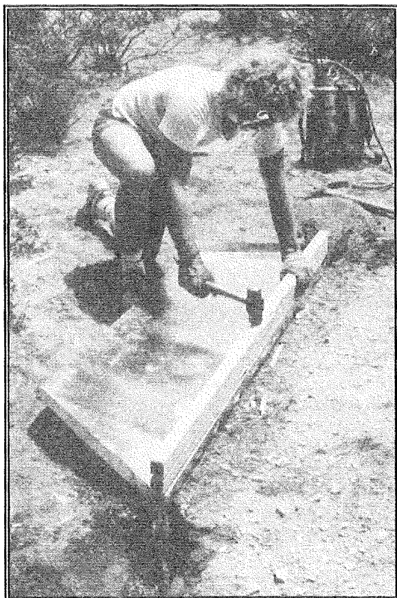
Runoff plots are installed in grass- and shrubland communities to examine the redistribution of water and nutrients as a function of vegetation type and rainfall.
