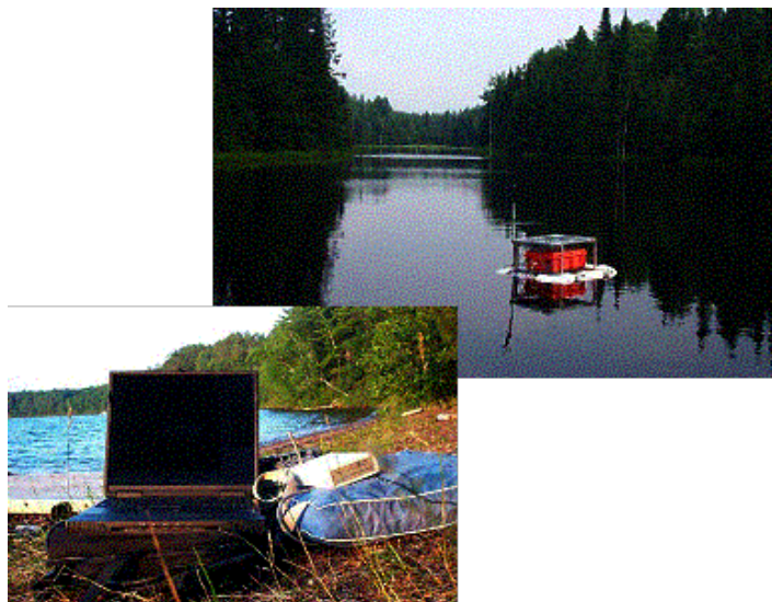
Figure 1. An example of serial spread spectrum communication between a laptop computer and a Campbell data logger located on a buoy.
