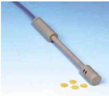
The FOXY (for Fiber Optic oXYgen sensor) unit operates by using a 470 nm light in
