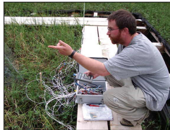
Neville Millar installing soil sensors in the Alaska Peatland Experiment, which looks at peatland carbon cycling through a series of water and thermal experiments. Photo: Molly Conlin.
