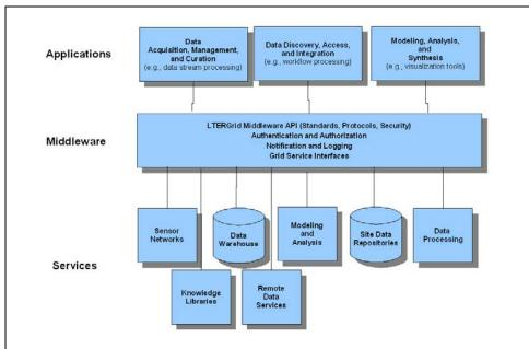
Figure 4. Schematic of Service-Oriented Architecture (SOA). Communication and security are standardized to present common interfaces to all data for service providers and consumers.
