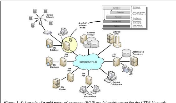
Figure 5. Schematic of a grid point-of-presence (POP) model architecture for the LTER Network
