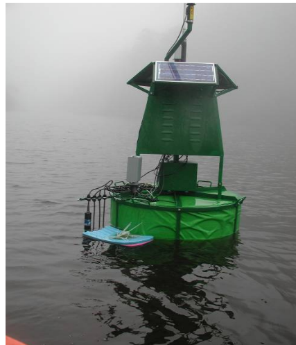
A buoy with the team’s sensors in the middle of Yuan Yang Lake, collecting data about dissolved oxygen, barometric pressure, wind speed, and temperature at various lake depths.
