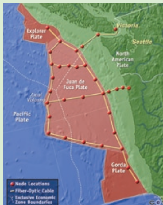
Figure 1. Cable Node Highlights: NEPTUNE’s 3,000-km network of fiber-optic/power cables will encircle and cross the Juan de Fuca tectonic plate. Between 30 and 50 experimental sites will be established at nodes along the cable and will be instrumented to interact with physical, chemical, and biological phenomena that operate across multiple scales of space and time. Node locations shown here are hypothetical. Final decisions on placement will depend on science input and engineering considerations.
