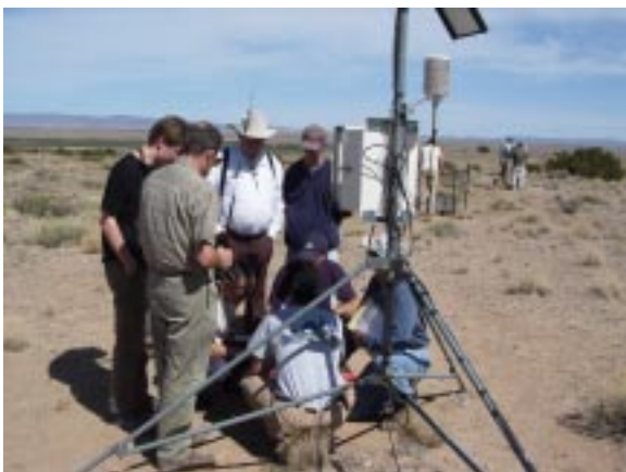
Workshop participants taking their final exam; hooking up a spread spectrum radio to the MET station to transmit data to a receiver located inside the Sevilleta. Note: Dave Hughes has his hands in his pockets (Photo: Pablo Bryant).
