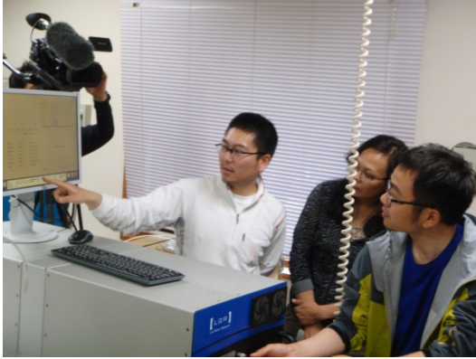
Photo 3. Group work for lab analysis using the Los-Gatos Isotopic N_2O Analyzer to measure N_2O concentration, stable isotope composition and isotope site preference.
