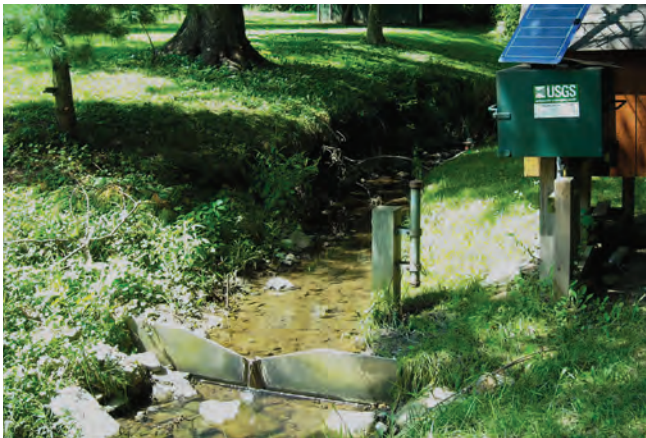
Long-term stream discharge and water chemistry site. Discharge is monitored in collaboration with the USGS and water samples are collected weekly by BES researchers. Image: Dan Dillon
