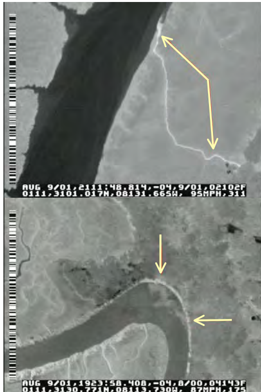
Fig. 2-12. Thermal images of Moses Hammock showing groundwater discharge. Freshwater appears white because it is cold. Top: Surficial groundwater flow at edge of Moses Hammock. Bottom: Sub-marsh groundwater inputs along the bend of a tidal creek.
